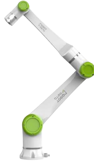
RM 1470/8 C Payload: 8 kg | Reach: 1468 mm
