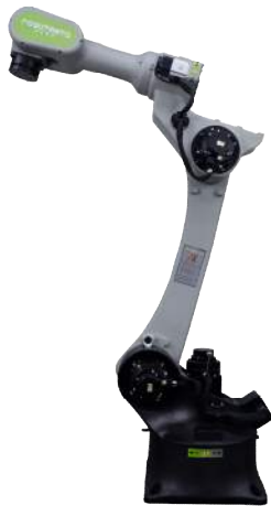
RM 1470/12 Payload: 12 kg | Reach: 1470 mm
