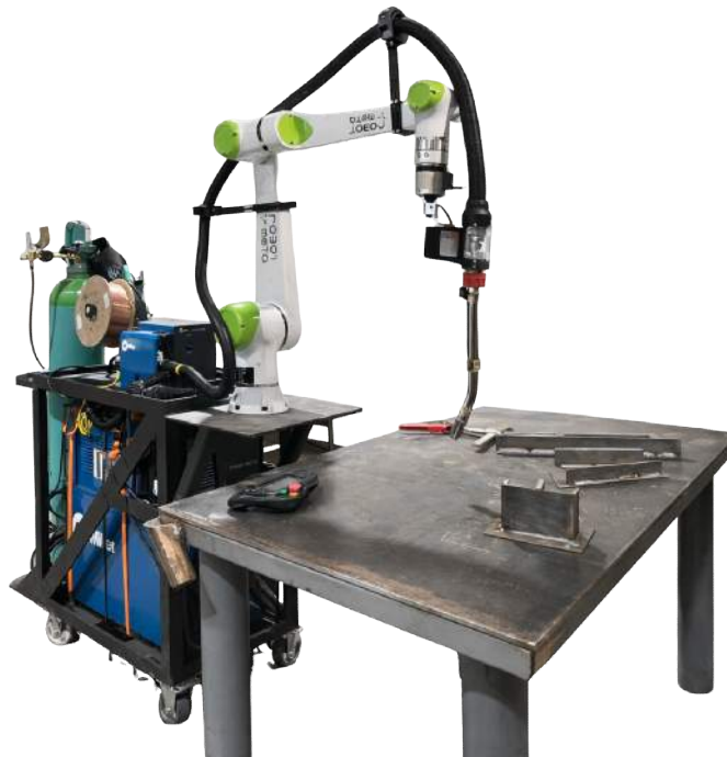
Mobile Welding Cart Setup
