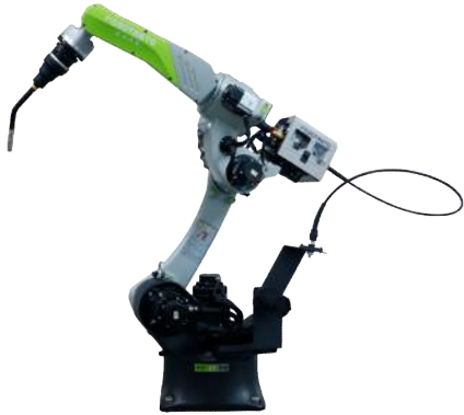
RM 1470/10 HW Payload: 10 kg | Reach: 1470 mm
