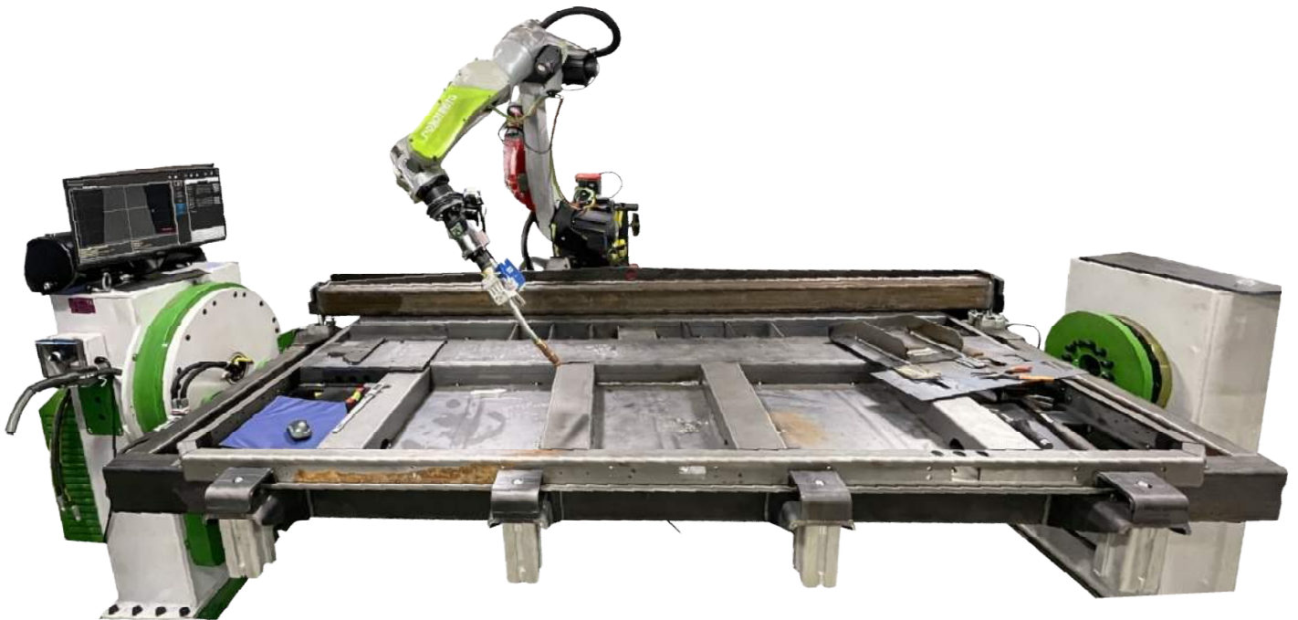
RM2000 with 2000kg 1-Axis Positioner
